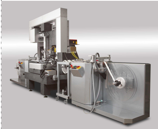
Fig. 3: LPKF-Laser equipment (reel-to-reel)
