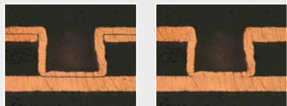
Detached layers from the activation step are reliably eliminated in the via-cleaning step.
