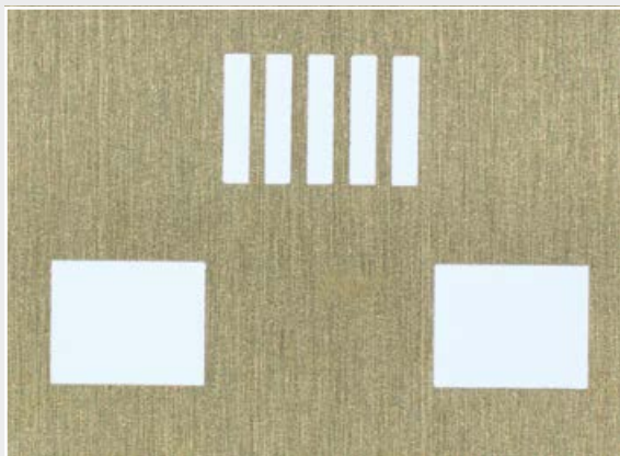
Easy processible SMT stencil from brass
