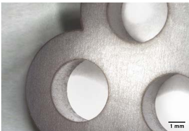
Up to 4-mm-thick stainless steel – low taper/sharp edges
